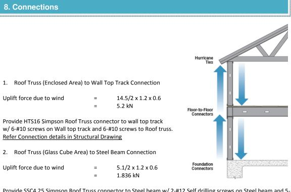
Provide SSC4.25 Simpson Roof Truss connector to Steel beam w/ 2-#12 Self drilling screws on Steel beam and 5-#10 screws to Roof truss.
