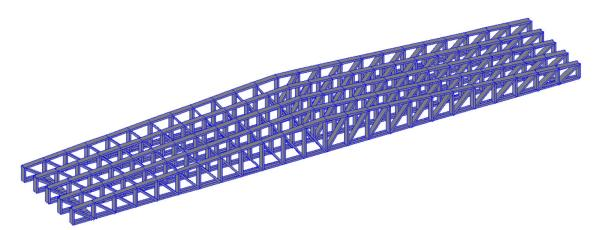
Refer Staad Analysis for Design Roof Truss, made up of Single 150S45-2.0 mm G350 at 600mm centre to centre.
